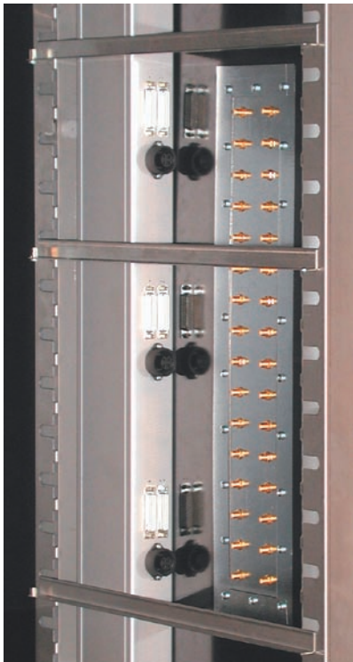
Interface connectors inside the chamber
